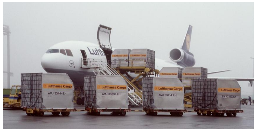
Loading of containers into an MD-11F of Lufthansa Cargo (Source: Wikipedia, GNU Free Documentation License, Author LCAG)
